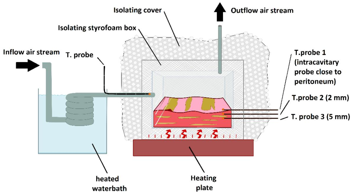
*Figure 7: Experimental abdominal box model. Abdominal cavity represented by a 4 litre styrofoam box with an additional isolation cover. Position of temperature sensors as illustrated.*
