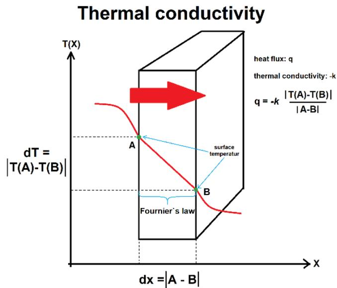
*Figure 2 Thermal conduction through a homogeneous material according to Fourier's law.  $q$  is the local heat flux density calculated by the material conductivity  $k$  and the temperature gradient.*
